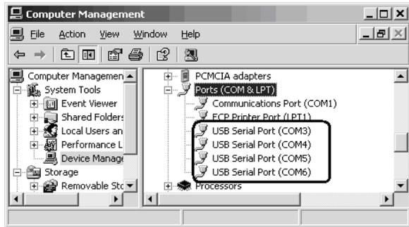
2. To view the RigExpert TI-5 serial port assignment, please run the **ListRE** program from **Start – Programs – RigExpert TI-5 – Show serial ports**:
