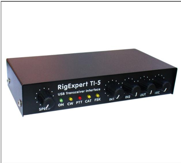
*RigExpert TI-5 is an electronic device designed to operate phone, CW, and digital modes using personal computer and transceiver. Previously, a TNC or sound card was needed for this purpose, along with lots of cables, occupying computer sound card and serial ports. All of this is not needed anymore. Following up-to-date technology, USB interface is chosen to connect RigExpert TI-5 to your computer. No additional interface circuit is needed for transceiver connection.*
