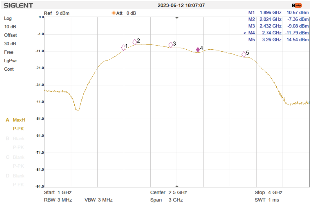
Figure 2. LNA Gain sweep. Input RF signal -40dBm
