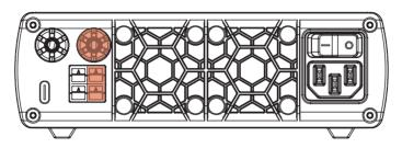
The loads can be connected also to Anderson Powerpole $^{\mathbb{R}}$  connectors at the rear panel. There are additional connectors at the rear panel of the power supply:
