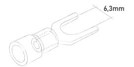
It is recommended to connect the load to the binding posts by Fork spade terminals.
