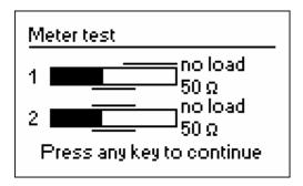
If the bars are not filled at all, the RF output stage or/and detectors are not working properly in the analyzer.
