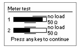
For the 50-Ohm load, the filled bars should stand at corresponding positions (notice the "no load" and "50  $\Omega$ " marks):
