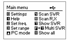
The *Main menu* contains a brief list of available commands. By pressing keys on the keypad, you may enter corresponding measurement modes, set up additional parameters, etc.
