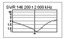
The above picture shows SWR graph of a vertical VHF antenna connected via a 40 m (131 ft) cable. The operating frequency is 146.2 MHz. The SWR at this frequency is about 1.1, which is acceptable.
