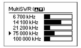
You may use this feature to tune multi-band antennas. Use the up and down cursor keys to select a frequency to be set or changed. Press the **0** key to switch between SWR bars and numerical representation of these parameters.
