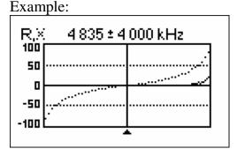
The 1/4-wave resonant frequency of the piece of open-circuited RG-58 cable is 4835 kHz
