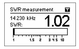
Set the desired frequency (the 2 key) or change it with left or right arrow keys.
