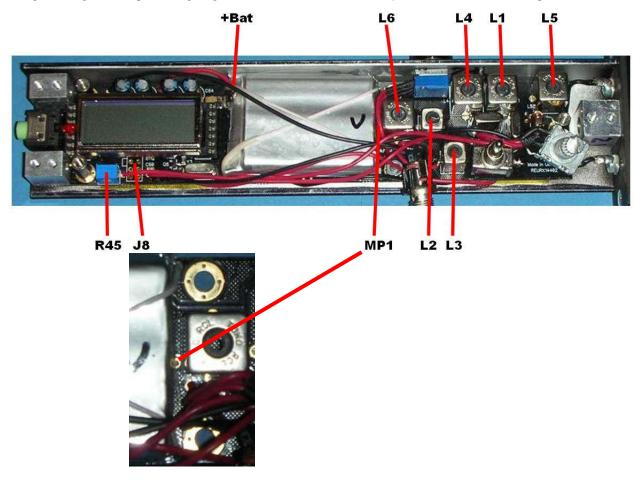
For the alignment of the receiver, the top L profile must be removed, as described above. Turn receiver on by plugging in the headphone.
