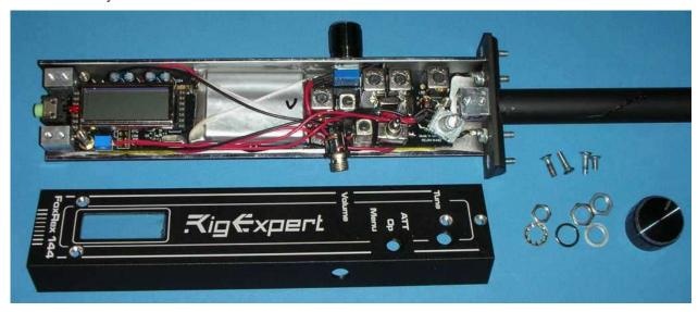
All components are mounted on a double-sided printed circuit board.
