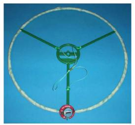
In order to get a defined omni-directional characteristic, I made a **ring dipole** (halo) out of the two antenna wires.
