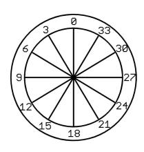
The FoxRex comes with a **compass mounted on the director boom**. It is not the fastest, but it finds the direction to (magnetic) North. If you want to read the headings to the fox directly, an **inverse scale** must be glued on, see the example above. The red end of the compass needle indicates the heading of the receiver's forward maximum (divided by 10).
