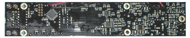
Above: The big circuit on the left is the Atmel processor, the RF/IF stages are on the right
