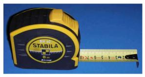
The material can be cut easily with old nail scissors. With a file you can round off the sharp edges. Drilling the holes in the spring steel is not easy, it tends to crack. I hold the tape measure between two wooden boards. It's best to make a few attempts first. RigExpert reinforces the elements in the center with a 40 cm long second layer, which is riveted at the ends. This is not absolutely necessary, but helps in case of strong wind or violent movements.
