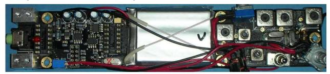
In the middle of the board you can see the Lithium-Polymer-accumulator, on the right side the RF and IF stages, and on the left side the display, processor and charger and voltage regulation circuits. The display is plugged into a socket and can be removed easily.
