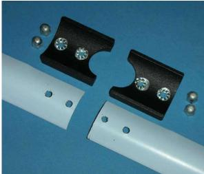
To remove the reflector (longest/rear element) unscrew two cap nuts, remove the narrow plate and reflector. See left photo. The large end plate is held by two countersunk screws. They must be removed only if you want to open the receiver.
