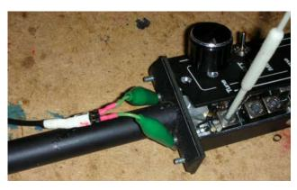
Connect a **signal generator** to the receiver, see the photo on the left. Remove the dipole (4 cap nuts) and connect the generator with a short adapter coax to 2 x mini crocodile clip.
