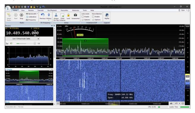
Now re-direct the output audio to your Virtual sound card. Run the WSJT-X software and set it up to receive from the same Virtual sound card. Now the FT-8 signals will be visible in the Wide Graph window:
