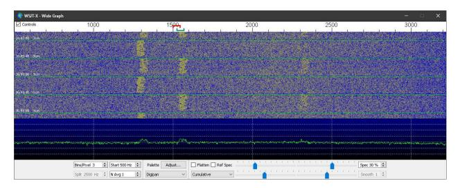
The WSJT-X software is now able to decode the FT-8 signals:
