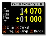
Press (Up) or (Down) cursor keys while holding the F (Functional) key to quickly choose a radio amateur band.
