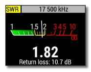
The SWR icon in the top-left corner flashes when the measurement is performed.
