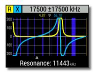
• If the value of X is moving from 0 to  $+\infty$ , the cable is short-circuited:
