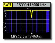
A one-turn coil (about 10 cm in diameter) connected to the analyzer was placed, co-axially, a few centimeters away from the measured trap. The SWR chart shows a visible dip at 17.46 MHz, which is a resonant frequency of the trap.
