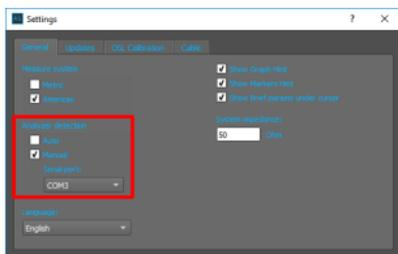
In the Antscope2 **Setup** window select the **Manual analyzer detection** checkbox and choose this port number.
