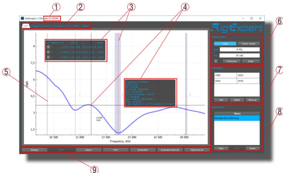
1. Window header. Connected analyzer model is shown here.
